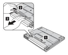
4. Install a fully charged battery.
