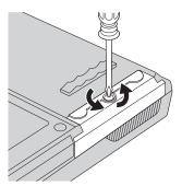
5. Open the computer display; then stand the computer on its side and remove the hard disk drive by pulling the cover away from the
