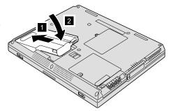
b) Slide the battery latch to lock it.
