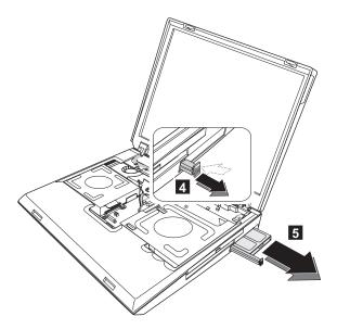
When installing: At steps 2 and 3, tighten the two new screws slowly until both screws have caught the first threads of the screw holes on the PC card slot assembly. Then, tighten each screw one turn at a time, alternating between screws to evenly pull the assembly connector onto the system board connector.
