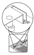
When Installing: Be sure the corners of the FDD cover go under the clasps on the FDD bracket.
