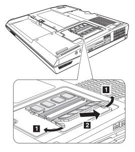
When installing: With the notched end of the DIMM toward the socket, insert the DIMM into the socket, and then press it firmly. Pivot the DIMM until it snaps into place. Make sure that the card is firmly fixed in the slot and does not move easily.
