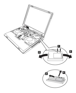
Removing and replacing a FRU
