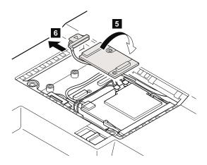
When installing: Make sure that connectors 4 and 6 are firmly attached.
