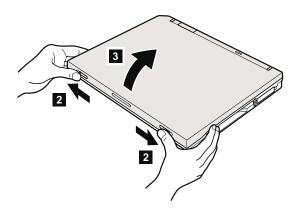
In step **5**, open the keyboard slightly in the direction of the arrow.
