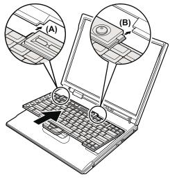
3. Press the keys indicated by arrows to latch the keyboard firmly in place.
