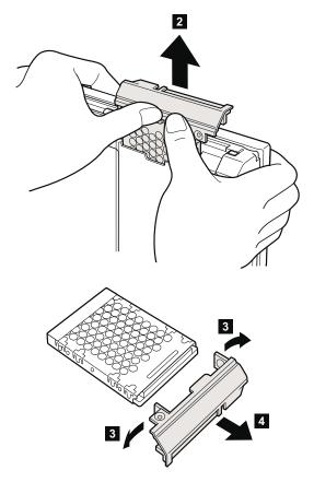
When installing: Make sure that the hard-disk connector is firmly connected.
