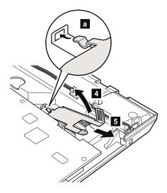
When installing: Do as shown in figure a .
