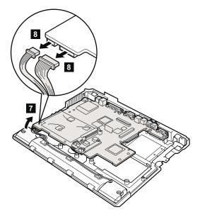
When installing: Make sure that both of the connectors are firmly attached.
