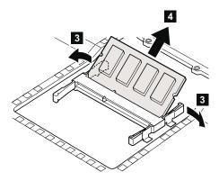
When installing: With the notched end of the DIMM toward the socket, insert the DIMM into the socket, and then press it firmly. Pivot the DIMM until it snaps into place. Make sure that the card is firmly fixed in the slot and does not move easily.
