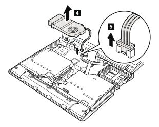
When installing: Make sure that the connector **5** is firmly attached.
