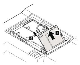
When installing: With the notched end of the card toward the socket, insert the card into the socket, and then press it firmly. Pivot the card until it snaps into place. Make sure that the card is firmly fixed in the slot and does not move easily.
