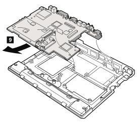
When installing: Attach the system board so that the two small projections on the base cover fit into the holes provided.
