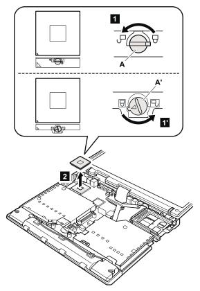
When installing: Place the CPU on the CPU socket (1), and then rotate the head of the screw (A) in the direction of arrow 2 to lock the CPU.
