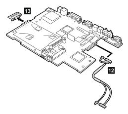
When installing: Make sure that the Ethernet/modem cable is firmly attached to two connectors on the bottom of the system board. And then, stick the EMI tape to secure the cable on the system board.
