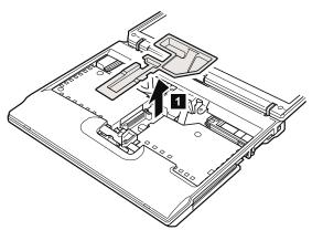
Keyboard CRU insulator **1a** is not fixed with an adhesive tape.
