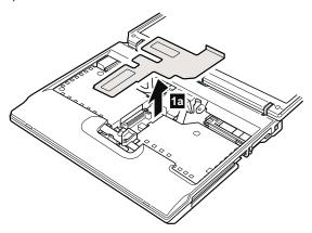
When installing: Some keyboard CRU insulators are not fixed with an adhesive tape and are easily moved. For those insulators, make sure that the keyboard CRU insulator is placed as in following figure. If the keyboard CRU insulator is not placed firmly, the keyboard cannot be installed properly.
