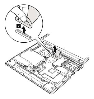
When installing: Make sure that the connector **2** is firmly attached.
