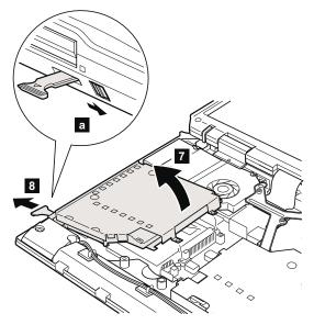
When installing: After inserting the Ultrabay release lever into the rectangular hole of base cover, slide the Ultrabay latch knob toward you until it snaps ( a ). Then attach the bay to the computer.
