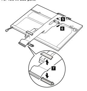
Cable routing: When installing the LCD, route the connector cable as in the following figure:
