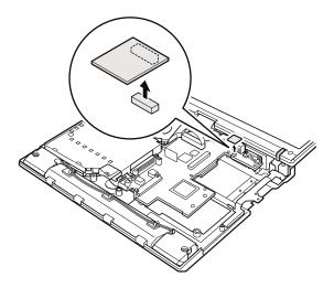
When installing: Make sure that the connector is firmly attached.
