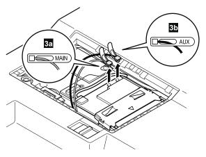
When installing: Plug the gray antenna cable with the tab marked "MAIN" (3a) into jack *J1*, and the black antenna cable with the tab marked "AUX" (3b) into jack *J2*.
