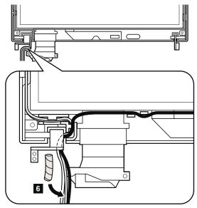
Slide the spiral tube in the direction of the arrow  $\cente{1}$ .
