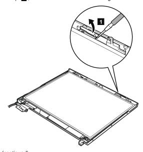
Lift the latch bar in the direction of the arrow 2, and then remove the left latch in the direction of the arrow 3.
