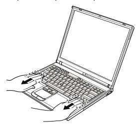
Make sure that all the projections on the front side of the keyboard b are firmly attached under the frame.
