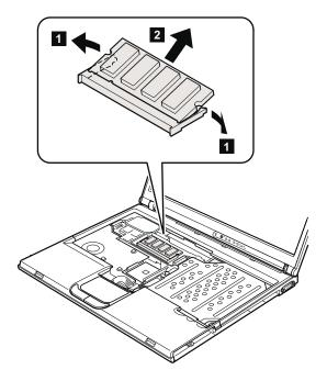
When installing: Insert the notched end of the DIMM into the socket. Press the DIMM firmly, and pivot it until it snaps into the place.
