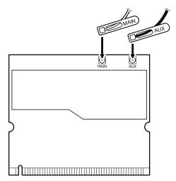
Insert the notched end of the card into the socket, and then press the card firmly. Pivot the card until it snaps into place. Make sure that it is firmly fixed in the slot and does not move easily.
