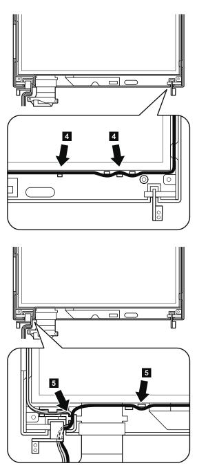
Coil the spiral tube round the antenna cables.
