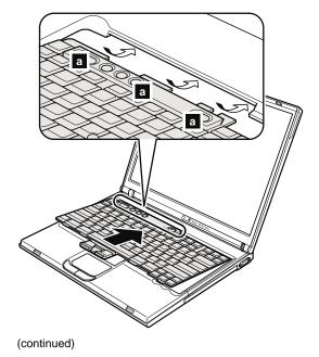
To make sure that the front side of the keyboard is housed firmly, gently press the keys with your fingers and try to slide the keyboard towards you.
