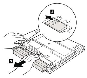
When installing: Install the battery pack along the slide rails on the left and right sides of the battery-pack slot. Make sure that both battery latches, a and b, are in the locked position, as in the following figure.
