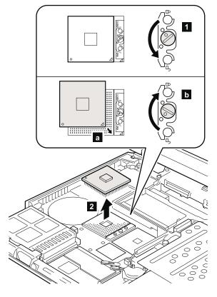
When installing: Place the CPU on the CPU socket a, and then rotate the head of the screw in the direction of arrow b to secure the CPU.
