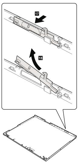
When installing: Attach the right latch to the LCD cover as follows:
