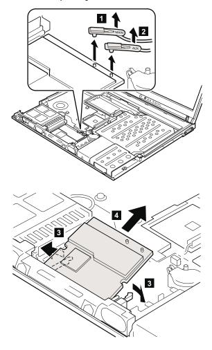
When installing: Plug in the wireless antenna cable as follows:
