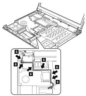
When installing: Make sure that the antenna cables are firmly routed as shown in the figure.
