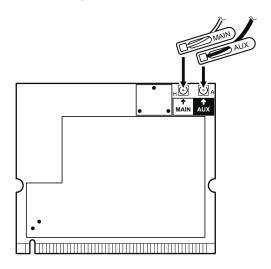
IBM Dual-Band 11a/b Wi-Fi Wireless Mini PCI Adapter Plug the gray antenna cable with the tab marked MAIN into jack MAIN, and the black antenna cable with the tab marked AUX into jack AUX.
