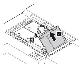
When installing: With the notched end of the card toward the socket, insert the card into the socket, and then press it firmly. Pivot the card until it snaps into place. Make sure that the card is firmly fixed in the slot and does not move easily. Removing and replacing a FRU
