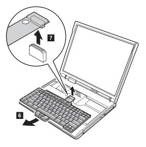
When installing: Install the new keyboard, following the directions below.
