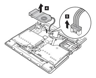
When installing: Make sure that the connector **5** is firmly attached.
