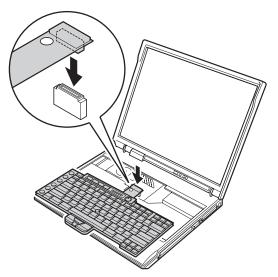
2. Make sure that the keyboard edges, shown in the figure as (A) and (B), are under the frame.
