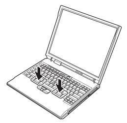
4. To make sure that the front side of the keyboard is housed firmly, insert your fingers into the left and right slots of the Ultrabay; then, with your fingers in those slots, gently press the shift keys with your thumbs and try to slide the keyboard towards you. Do not push hard on parts (A) and (B) on the keyboard; to do so might distort the Ultrabay slots.
