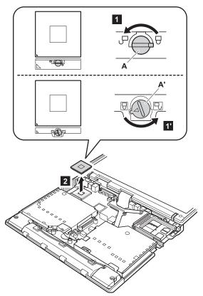
When installing: Place the CPU on the CPU socket (1), and then rotate the head of the screw (A) in the direction of arrow 2 to lock the CPU.
