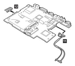
When installing: Make sure that the Ethernet/modem cable is firmly attached to two connectors on the bottom of the system board. And then, stick the EMI tape to secure the cable on the system board.
