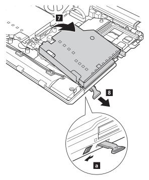
When installing: After inserting the Ultrabay release lever into the rectangular hole of base cover, slide the Ultrabay latch knob toward you until it snaps ( a ). Then attach the bay to the computer.
