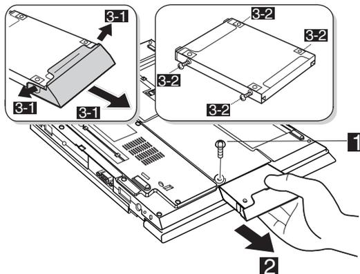
5. Remove the hard-disk drive by pulling the cover away from the computer (2).
