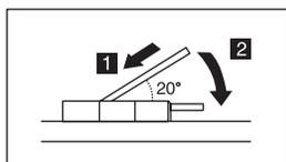
7. Pivot the DIMM until it snaps into place.
