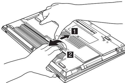
4. Align the side of a fully charged spare battery pack with the side of the battery space in the computer **1**; then gently push the battery into the
