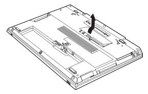
If the DIMM is already in the memory slot, remove it to replace the new one by pressing out on the latches on both edges of the socket at the same time. Be sure to save it for future use.
