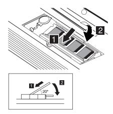
7. Pivot the DIMM until it snaps into place.
