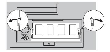
5. Find the notch on the side of the DIMM.
