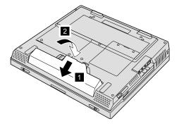
b) Slide the battery latch to lock it.
