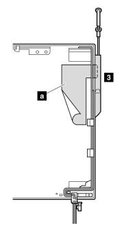
**When installing:** As you route the cables, make sure that they are not subjected to any tension. Tension could cause the cables to be damaged by the cable guides, or a wire to be broken.
