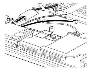
Then plug the gray cable into the jack labeled **MAIN**, and the black cable into the jack labeled **AUX** on the card.
