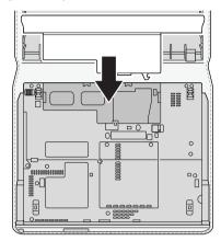
6. Slide the battery lock to the locked position.
