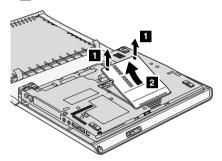
7. Remove one of two SO-DIMMs already installed to make room for the new one by pressing out on the latches on both edges of the socket at the same time. Be sure to save the old SO-DIMM for future use.
