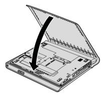
2. While holding the front side of the computer as shown in the drawing, pull the cover toward you and downward.
