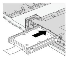
Reinstall the cover of the hard disk drive slot 1. Then, reinstall the screw 2.
