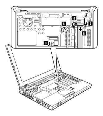
When installing: Make sure that all the connectors are attached firmly.
