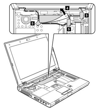
Release the antenna cables from the cable guides of the frame. In step 6, take care not to damage the cables when you pull out them from the guide hole.
