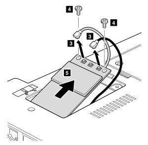
In step 3, unplug the jacks by using the removal tool antenna RF connector (P/N: 08K7159) or pick the connectors with your fingers and gently unplug them in direction of the arrow.
