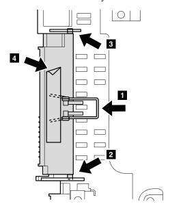
For PC Card/Smart Card slot bezel assembly
