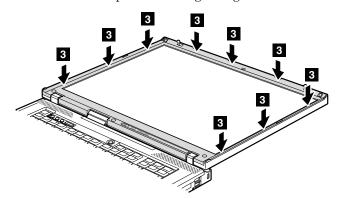
3. Attach the LCD rear cover from the top end.
