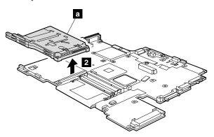
When installing: Make sure that the connector of the PC Card/Express Card slot assembly is attached to the system board firmly.
