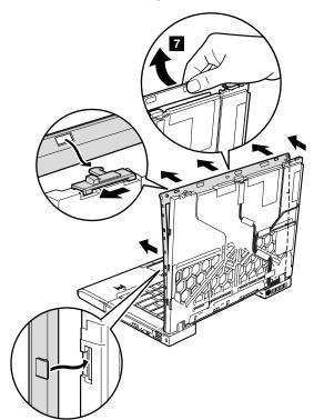
Detach the latches on the front edge of the LCD front bezel in the direction of arrow 8 as shown in this figure.
