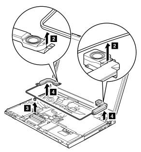
For Vodafone wireless WAN models: When replacing the speakers, reuse the ferrite core a that has been attached to the old FRU.
