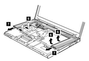
When installing: Make sure that all the claws are attached firmly.
