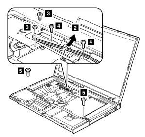
In step 2, release the wireless antenna cables from the cable guide.
