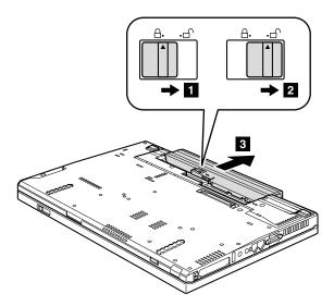
**When installing:** Install the battery pack along the slide rails of the slot. Then make sure that the battery release lever is in the locked position.
