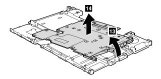
When installing: For the models with the wireless WAN features, you need to attach the cushion attach the cushion that is shipped with new structure frame. Peel off the covering film of the adhesive tape on bottom side of the cushion, and paste it on the new structure frame as shown in this figure.
