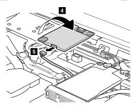
**When installing:** Make sure that the modem connector and the connector on the underside of the card are attached firmly.
