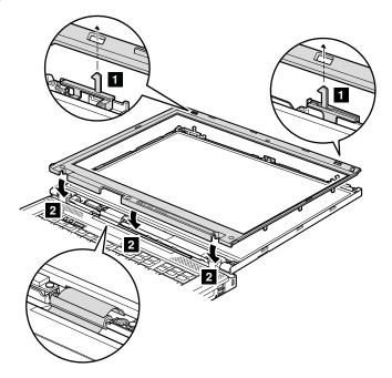
2. Attach all the latches on the top, left, and right edges of the bezel.
