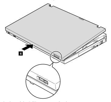
4. Attach the latches of the LCD rear cover firmly.
