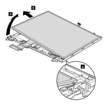
When installing: Attach the LCD panel so that the small hole on the right side of the panel fits into the small projection of the right hinge as shown in **a**.
