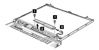
When installing: Make sure that connectors 3 and 4 are attached firmly.
