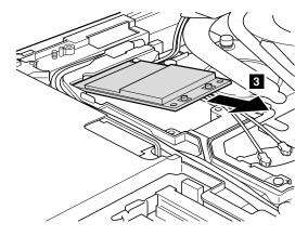
Cable routing: When you install the the card, route the antenna cables as shown in this figure.
