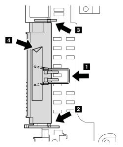
For PC Card/Smart Card slot bezel assembly
