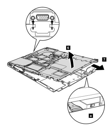
When installing the PC Card slot bezel assembly, do as follows:
