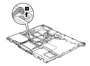
When installing: Make sure that the speaker connector is attached firmly.
