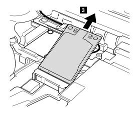
When installing: Plug the gray cable into the jack labeled MAIN on the card, and the black cable into the jack labeled AUX.
