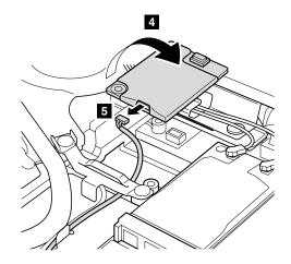
Turn the card over  $\ensuremath{4}$  , and detach the modem connector  $\ensuremath{5}$  .
