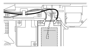
Some ThinkPad computer has three cables and the 802.11 a/b/g/n wireless LAN card. In that case, plug the gray cable (MAIN) into the jack labeled **TR1**, the white cable (3rd) into jack labeled **R0**, and the black cable (AUX) into jack labeled **TR2** on the card.
