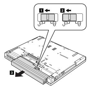
**When installing:** Install the battery pack along the slide rails of the slot. Then make sure that the battery release lever is in the locked position.
