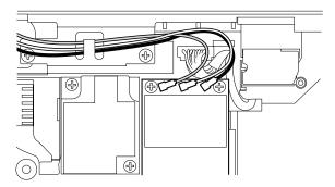
After you secure the card, make sure that the antenna cables are routed as shown in the each figure.
