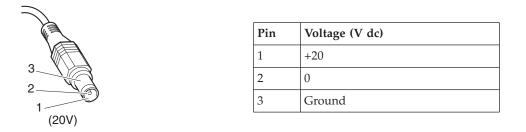
**Note:** Output voltage of pin no.2 of the ac adapter may different from the one you are servicing.
