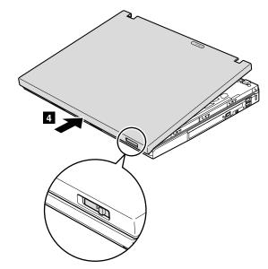
4. Attach the latches of the LCD rear cover firmly.
