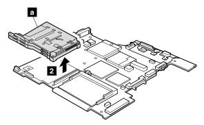
When installing: Make sure that the connectors of the PC Card/Express Card slot assembly and of the interposer card are attached to the system board firmly.
