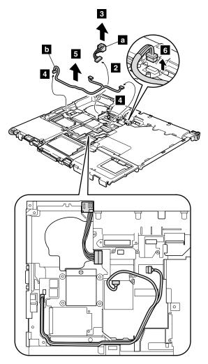
Remove the ac power jack cable **a** and the modem cable **b**.
