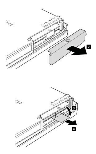
When installing: Make sure that the hard disk drive connector is attached firmly.
