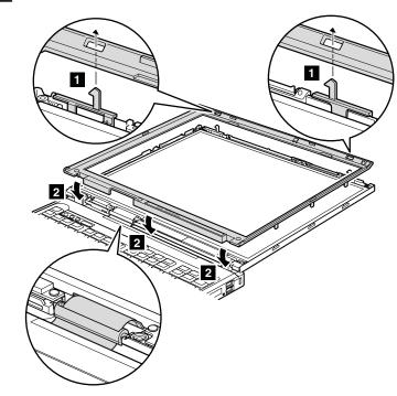
2. Attach all the latches on the top, left, and right edges of the bezel.
