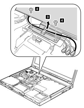
In step **3** , release the wireless antenna cables from the cable guide.
