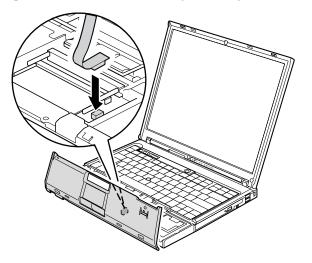
2. Press the left and right top edges of the palm rest to fit it into place.
