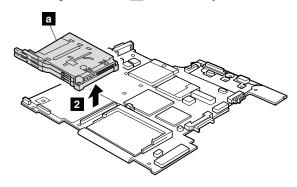
When installing: Make sure that the connectors of the PC Card/Express Card slot assembly and of the interposer card are attached to the system board firmly.
