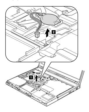
When installing: Make sure that the battery connector is attached firmly.
