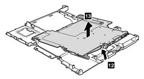
When attaching the system board to the frame, do as follows:
