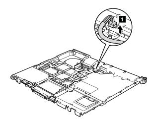
**When installing:** Make sure that the connector **1** is attached firmly.
