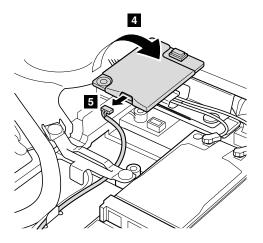
When installing: Make sure that the modem connector and the connector on the underside of the card are attached firmly.
