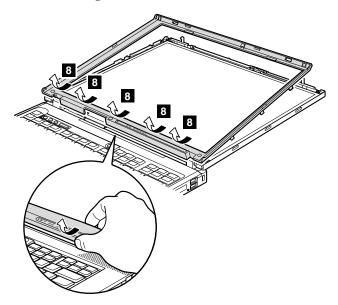
When installing: Attach the LCD cover kit as follows:
