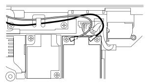
If the computer you are servicing has three cables and the 802.11 a/b/g wireless LAN card, put the white cable in the cable bag in the card slot.
