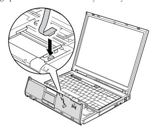
2. Press the left and right top edges of the palm rest to fit it into place.
