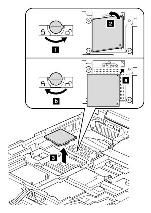
When installing: Place the CPU on the CPU socket **a**, and then rotate the head of the screw in the direction shown by arrow **b** to secure the CPU.
