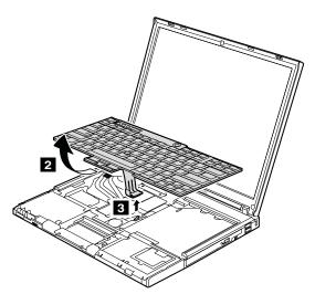
When installing: Make sure that the keyboard edges a are under the frame as shown in this figure.
