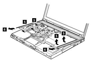
When installing: Make sure that all the claws are attached firmly. Then fasten the screws to secure the keyboard bezel.
