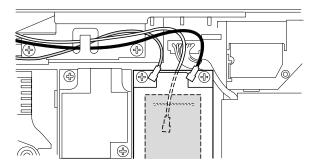
Some ThinkPad computer has three cables and the 802.11 a/b/g/n wireless LAN card. In that case, plug the gray cable (MAIN) into the jack labeled  $\mathbf{TR1}$ , the white cable (3rd) into jack labeled  $\mathbf{R0}$ , and the black cable (AUX) into jack labeled  $\mathbf{TR2}$  on the card.
