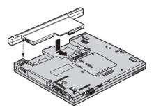
6. Slide the battery lock to the locked position.
