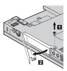
5. Remove the hard disk drive by pulling out the tab.
