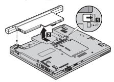
5. Install a fully charged battery.
