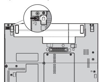
6. Slide the battery lock to the locked position.
