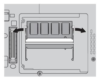
7. With the notched end of the SO-DIMM toward the contact edge side of the socket, firmly insert the SO-DIMM into the socket at an angle of about 20 degrees 1; then pivot it downward until it snaps into place 2.
