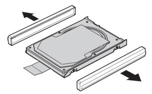
7. Attach the side rubber rails to a new hard disk drive.
