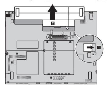
5. Install a fully charged battery.
