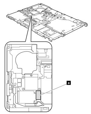
2. For the models with Sierra Wireless EV-DO Wireless WAN Mini PCI Express Adapter, you need to attach the shield sheet that is shipped with new structure frame. Peel off the covering film of the adhesive tape on bottom side of the shield sheet, and paste it on the new structure frame as shown in this figure.
