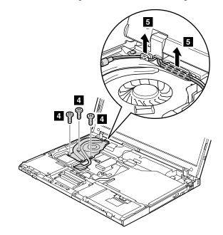
**Attention:** Do not handle the fan roughly. Improper handling of the fan can cause distortion or deformation and imperfect contact with components.
