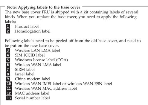
For some models, you also need to apply one or two FCC labels. Check the old base cover; if it has one or two FCC labels, find duplicates of them in the label kit and apply them to the new base cover.
