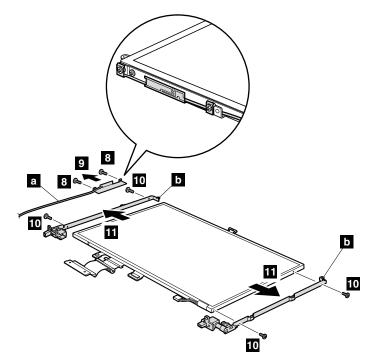
In steps **8** and **9**, remove the wireless LAN 3rd antenna (**a**) from the left hinge.
