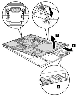
Attention: Before step **7**, be sure that the Ultrabay Slim device eject lever has not popped out. It must be housed in its position as shown in the figure **a**.
