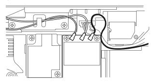
When installing: Plug the gray cable (MAIN) into the jack labeled **TR1**, the white cable (3rd) into jack labeled **R0**, and the black cable (AUX) into jack labeled **TR2** on the card.
