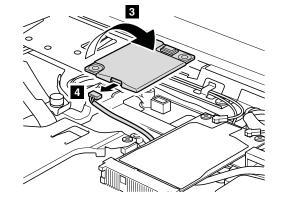
Turn the card over 3, and detach the modem connector 4.
