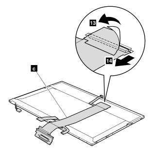
Remove the LCD cable assembly ( **c** ) from the LCD panel.
