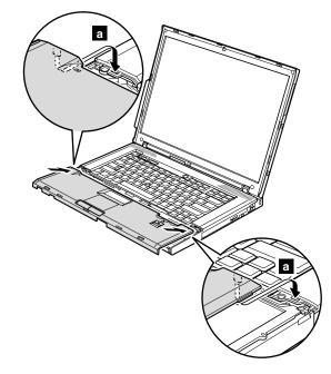
**3**. Align the front side of the palm rest to the frame, and press the front edge to latch the palm rest to the frame as shown in this figure.
