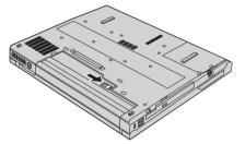
6. Turn the computer over again. Connect the ac adapter and the cables to the computer.
