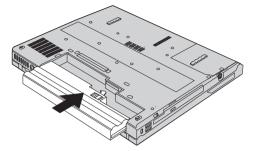
5. Slide the battery latch to the lock position.
