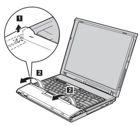
**Note:** When you lift the left and front edges of the palm rest, it is normal to hear a click.
