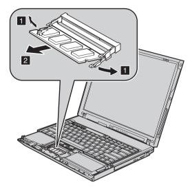
11. With the notched end of the SO-DIMM toward the contact edge side of the socket, firmly insert the SO-DIMM into the socket at an angle of about 20 degrees 1; then pivot it downward until it snaps into place 2.
