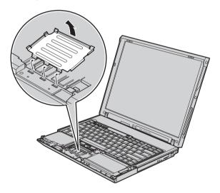
10. If two SO-DIMMs are already installed in the memory slot, remove one of them to make room for the new one by pressing out on the latches on both edges of the socket at the same time 1. Be sure to save it for future use 2.
