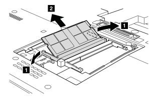
When installing: Insert the notched end of the DIMM into the socket. Press the DIMM firmly, and pivot it until it snaps into the place. Make sure that it is firmly fixed in the slot and does not move easily.
