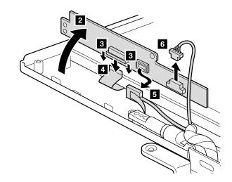
When installing: Make sure that connectors **4** , **5** , and **6** are attached firmly.
