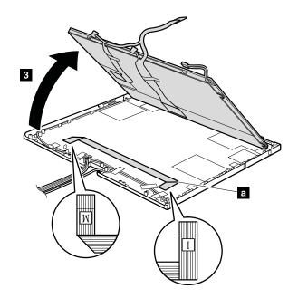
When installing: Place the FFC ( a ) on the rear cover of the LCD, in the direction shown in the figure above.
