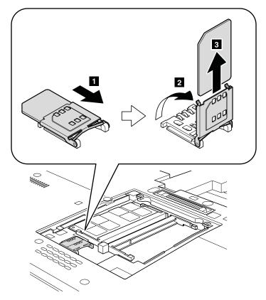
If the SIM card has been inserted in its slot, remove it before you start the servicing.
