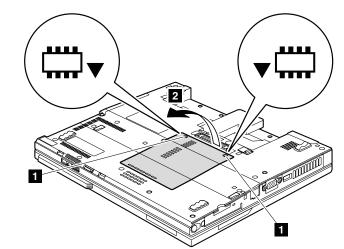
Remove the DIMM as shown in this figure.
