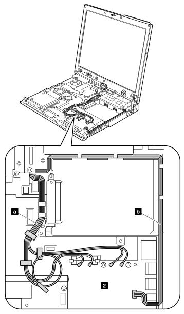
When installing: Make sure that the cables are routed as shown in this figure.
