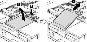
When installing: Plug the gray cable 1a into the jack labeled MAIN on the card, and the black cable 1b into the jack labeled AUX. If the computer you are servicing has three cables, put the white cable in the cable bag in the card slot.
