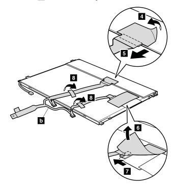
**When installing:** Make sure that the connectors of the LCD cable are attached firmly.
