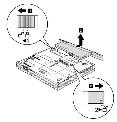
**When installing:** Install the battery pack along the slide rails of the slot. Then make sure that the battery release lever is in the locked position.
