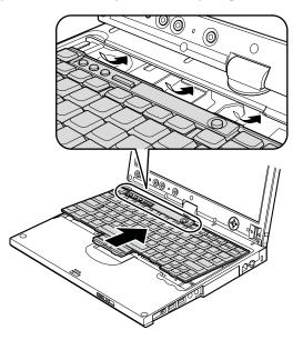
**3**. To make sure that the front side of the keyboard is housed firmly, gently press the keys with your thumbs and try to slide the keyboard toward you.
