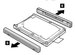
**When installing:** The rubber rails on the hard disk drive must be attached to the replacement drive. Otherwise the drive cannot be installed properly.
