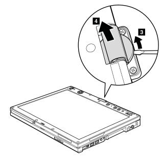
Before removing the hinge cap (small) in step **5**, rotate the LCD unit back to the original position, and close the LCD cover.
