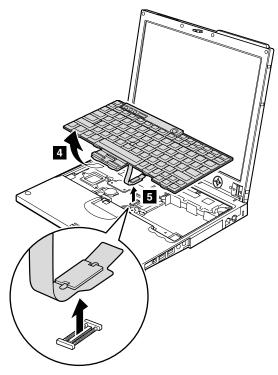
Lift the keyboard a little in the direction shown by arrow [4], and then detach the connector [5].
