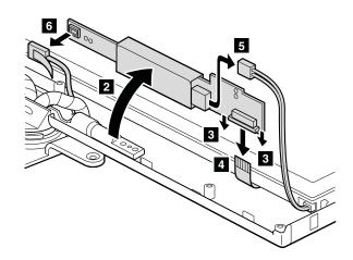
When installing: Make sure that connectors **4** , **5** , and **6** are attached firmly.
