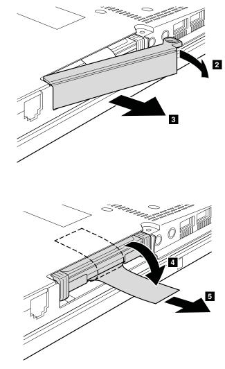
Remove the hard disk drive slot cover in step **2** and **3**.
