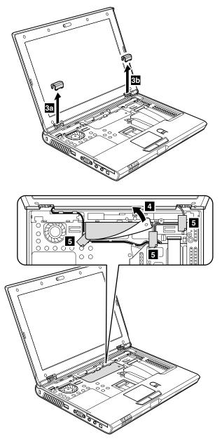
Release the antenna cables from the cable guides of the frame. In step 6, take care not to damage the cables when you pull out them from the guide hole.
