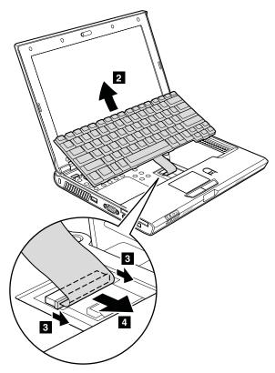
Lift the keyboard a little in the direction shown by arrow 2. Then unlock the connector 3 and detach the connector 4.
