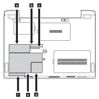
For some models, you also need to apply one or two FCC labels or the other types of labels. Check the old base cover; if it has one or two FCC labels or the other types of labels, find duplicates of them in the package and apply them to the new base cover.
