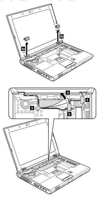
Release the antenna cables from the cable guides of the frame. In step 6, take care not to damage the cables when you pull out them from the guide hole.
