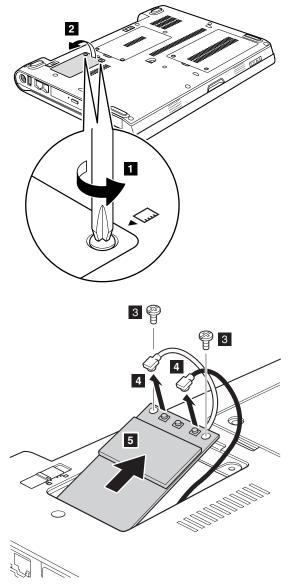
In step 3, unplug the jacks by using the removal tool antenna RF connector (P/N: 08K7159) or pick the connectors with your fingers and gently unplug them in direction of the arrow.
