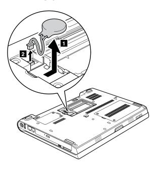
When installing: Make sure that the battery connector is attached firmly.
