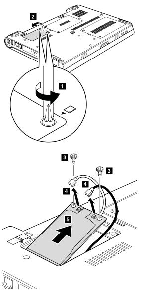
In step 3, unplug the jacks by using the removal tool antenna RF connector (P/N: 08K7159) or pick the connectors with your fingers and gently unplug them in direction of the arrow.
