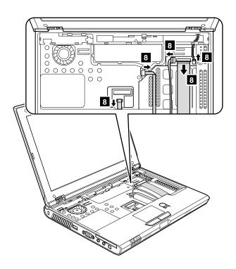
When installing: Make sure that all the connectors are attached firmly.
