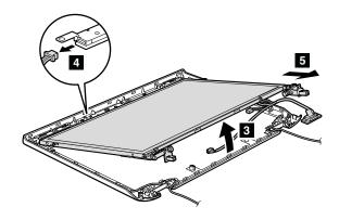
When installing: Make sure that the camera connector is attached firmly.
