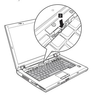
When installing: Make sure that the latch is attached firmly. Then secure the screws.
