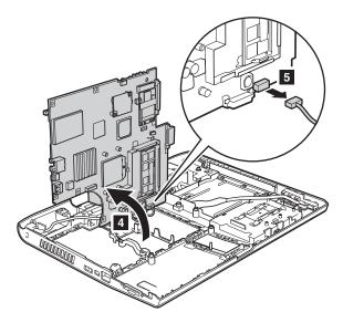
In step 4, remove the system board, the MDC, and the PC Card slot together from the bottom cover, and then detach the VGA connector 5.
