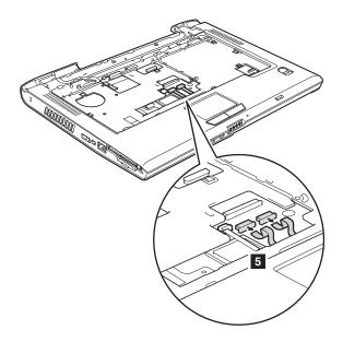
When installing: Make sure that the connectors are attached firmly.
