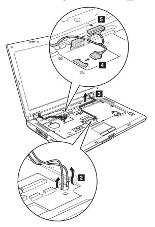
When installing: Make sure that the connectors 4 and 5 are attached firmly. (continued)
