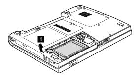
When installing: Make sure that the hard disk drive connector is attached firmly.
