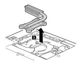
When installing: Before you attach a new thermal module to the computer, peel off the covering film of thermal grease. Then attach the thermal module to the computer.
