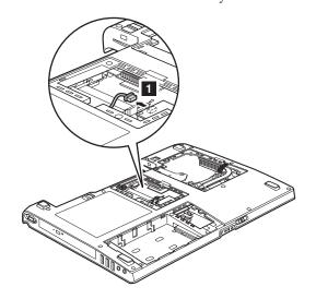
When installing: Make sure that the connectors are attached firmly.
