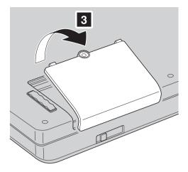
Remove the hard disk by pulling out the tab. ThinkPad Z61t
