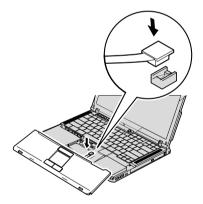
11. Align the front side of the palm rest with the front edge of the system1 , then put down the palm rest to replace it2 .
