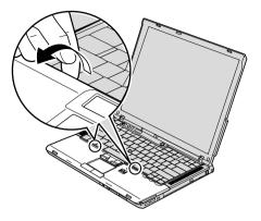
7. Move the palm rest carefully away from the computer until you can see where it's connected 1, and then detach the connector 2. Now the palm rest has been removed.
