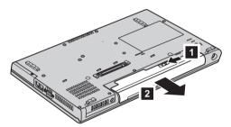
4. Install a fully charged battery.
