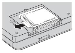
6. Detach the side rubber rails from the hard disk drive.
