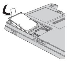
Align the front side of the hard disk cover 1, reinstall the cover 2, and tighten the screws 3.
