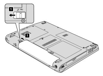
4. Unlock the battery latch 2 by sliding it to the unlocked position, and while holding it in the position remove the battery 3.
