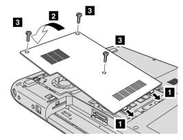
**Attention:** When you have added or upgraded an SO-DIMM, do not use your computer until you have closed the memory slot cover. Never use the computer with the cover open.
