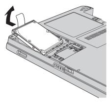
6. Place a new hard disk drive into the hard disk drive bay, then connect it firmly .
