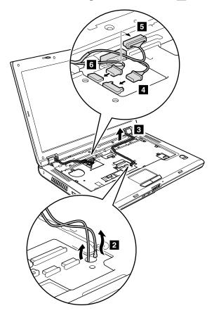
When installing: Make sure that the connectors 4, 5, and 6 are attached firmly.
