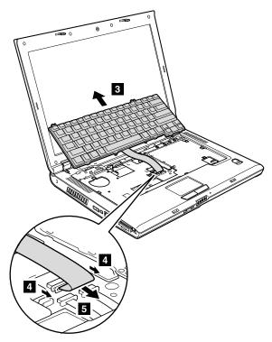
**When installing:** Make sure that the keyboard connector is attached firmly. Then lock the connector.
