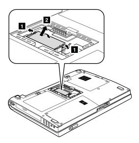
When installing: Insert the notched end of the DIMM into the socket. Press the DIMM firmly, and pivot it until it snaps into the place. Make sure that it is firmly fixed in the slot and does not move easily.
