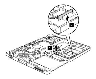
When installing: Make sure that the connector is attached firmly.
