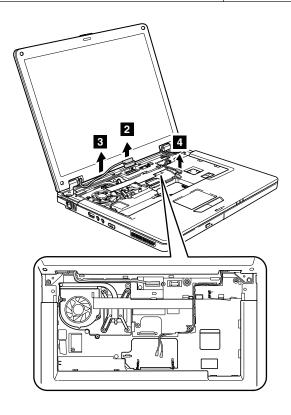
When installing: Make sure that the LCD connector is attached firmly.
