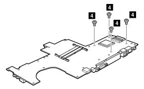
Turn over the system board again, and then remove the PC Card slot assembly.
