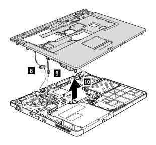
When installing: Make sure that the connectors 8 and 9 are attached firmly.
