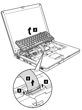
**When installing:** Make sure that the keyboard connector is attached firmly. Then lock the connector.
