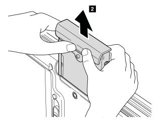
When installing: Make sure that the hard disk drive connector is attached firmly.
