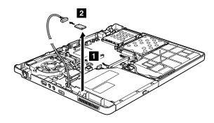
When installing: Make sure that connector is attached firmly.
