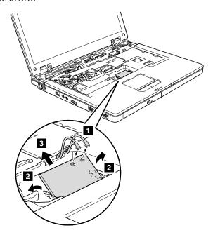
When installing: Plug the black cable into the jack labeled MAIN on the card, and the white cable into the jack labeled AUX.
