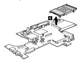
When installing: Make sure that the connectors of PC Card slot assembly is attached to the system board firmly.
