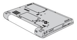
4. Unlock the battery latch 2 by sliding it to the unlocked position. While holding the latch in the unlocked position, remove the battery 3.
