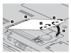
**Attention:** When you have replaced the SO-DIMM, do not use your computer until you have closed the memory slot cover. Never use the computer with the cover open.
