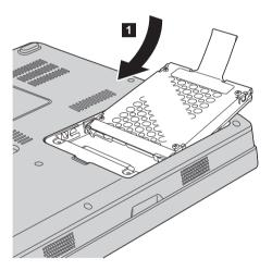
7. Reinstall the cover by aligning the front side of the cover first 1, and closing the cover 2. Then tighten the two screws 3.
