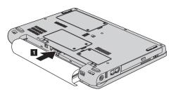
6. Slide the battery latch to the locked position 2.
