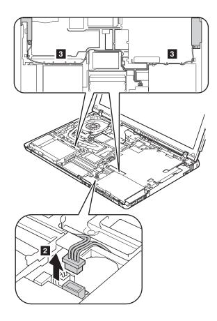
When installing: Make sure that the speaker cables are routed along the cable guides 3 and that the connector 2 is attached firmly.
