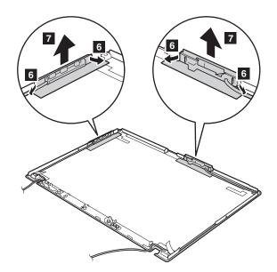
Cable routing: Route and secure the antenna cables as shown in the following figures.
