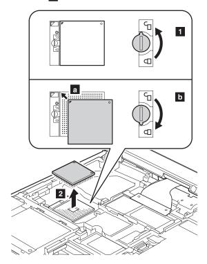
When installing: Place the CPU on the CPU socket **a**, and then rotate the head of the screw in the direction shown by arrow **b** to secure the CPU.
