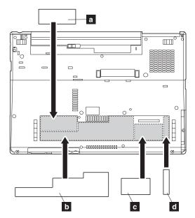
For some models, you also need to apply one or two FCC labels or the other types of labels. Check the old base cover; if it has one or two FCC labels or the other types of labels, find duplicates of them in the package and apply them to the new base cover.
