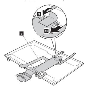
When installing: When replacing any LCD FRUs, be sure not to pinch the antenna cables. Make sure that the cables are routed as shown in the figures on page 113 and 114.
