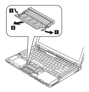
When installing: Insert the notched end of the DIMM into the socket. Press the DIMM firmly, and pivot it until it snaps into the place. Make sure that it is fixed firmly in the slot and does not move easily.
