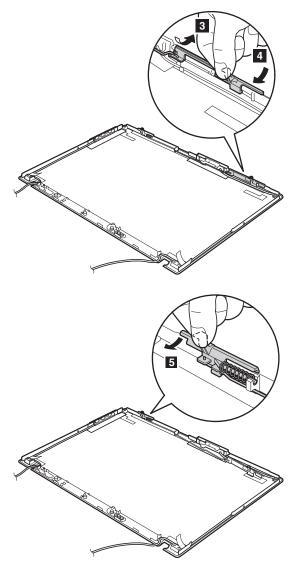
When installing: Attache the latches as shown in this figure.
