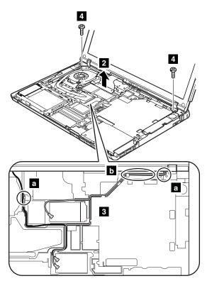
In step **3**, release the antenna cables from the cable guides.
