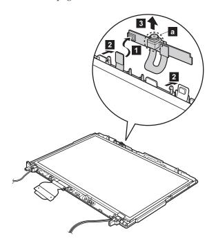
**Note:** The part marked **a** is fragile and easy to break. When you deal with the camera assembly, do not hold that part to avoid damage.
