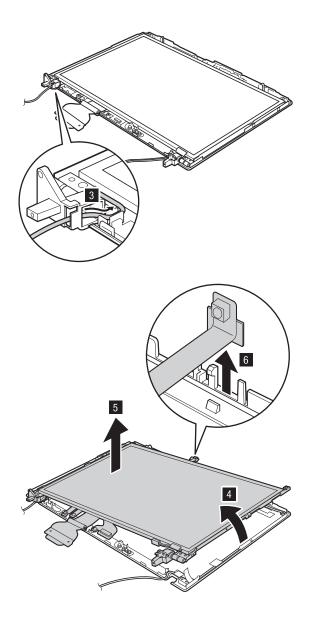
Remove the hinges **a** from the LCD panel.
