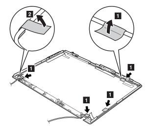
Remove the LCD latches before you remove the antenna cables.
