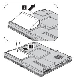
4. Align the front of a fully charged battery with the computer first and press firmly until you hear a click.
