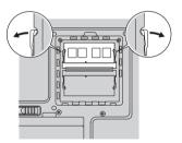
7. With the notched end of the SO-DIMM toward the contact edge side of the socket, firmly insert the SO-DIMM into the socket at an angle of about 20 degrees; then pivot it downward until it snaps into place.
