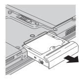
6. Insert a new hard disk drive into the hard disk drive bay firmly; then tighten the screw.
