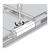
5. Remove the hard disk by pulling the cover.
