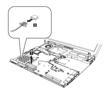
When installing: Make sure that the speaker connector is attached firmly.
