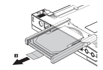
When installing: Make sure that the hard disk is connected firmly.
