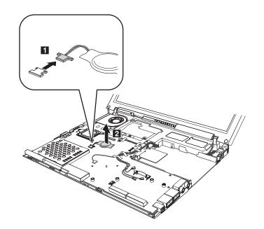
When installing: Make sure that the battery connector is attached firmly.
