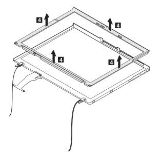
**When installing:** The replacement bezel should have adhesive pre-applied; therefore, remove the covering from the bezel to expose the adhesive, and then place the top edge under the frame, then push the bezel down and secure with the latches firmly. Be careful to route the antenna cables properly.
