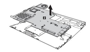
When installing: Do not damage the wireless micro switch 1 on the system board.
