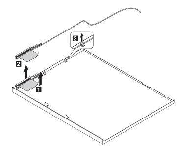
**Note:** For models with wireless WAN, the antennas present on the right-side are the aux wireless LAN antenna and the main wireless WAN antenna.
