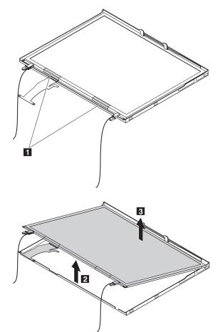
**When removing:** Make sure you do not touch or put pressure on these two sections of the LCD indicated below.
