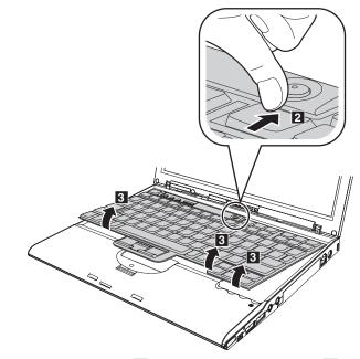
Detach the keyboard connector 4 to remove the keyboard 5.
