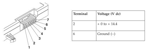
**3**. If the voltage is less than +14.4 V dc, the battery pack has been discharged.
