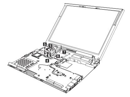
When installing: Make sure to position the LCD cable properly and reattach the mylar and tape. The LCD cable switch should fit in its slot **7**.
