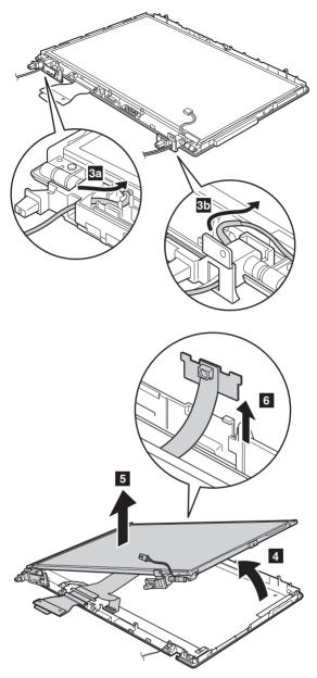
Remove the hinges ( a ) from the LCD panel.
