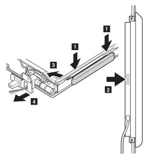
Note: In step 4, do not tense the cable. To do so, the cable may get damaged by the hinge, and may cause a broken wire.
