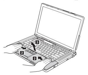
Pull the palm rest a little in the direction shown by arrow , and then detach the touch pad connector by pulling the tab with your fingers in the direction shown by arrow .
