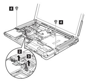
Strip the tape that secures the cable  $\begin{tabular}{|c|c|c|c|c|} 2 \\ \hline \end{tabular}$  , and disconnect the speaker cable  $\begin{tabular}{|c|c|c|c|} 3 \\ \hline \end{tabular}$  .
