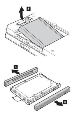
When installing: Rubber rails of the hard disk drive must be attached to the replacement drive. Otherwise the hard disk drive cannot be properly installed to the computer.
