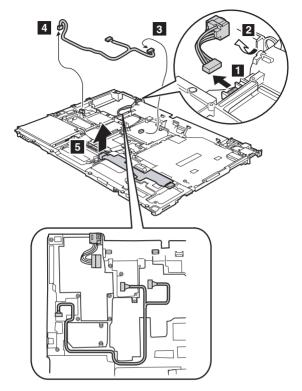
When installing: Make sure the connectors are attached firmly, and that the cables are routed as in the figure above.
