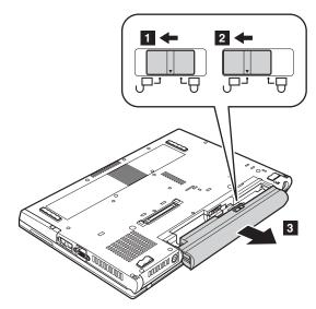
**When installing:** Install the battery pack along the slide rails of the slot. Then make sure that the battery release lever is locked, as in this figure.
