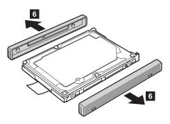
**When installing:** Rubber rails of the hard disk drive must be attached to the replacement drive. Otherwise the hard disk drive cannot be properly installed to the computer.
