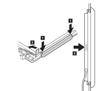
When installing: In step **2**, press the part indicated by the arrow until it snaps into place.
