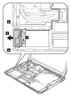
**When installing:** Make sure that the antenna cable is routed along the cable guides, and that the antenna is attached to the guides **a** firmly.
