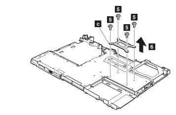
Remove the CPU support plate **c**.
