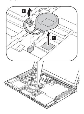
When installing: Make sure that the battery connector is attached firmly.
