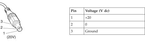
**Note:** Output voltage of pin no.2 of the ac adapter may different from the one you are servicing.
