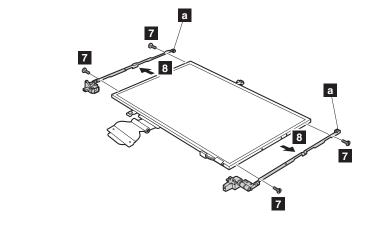
Remove the hinges **a** from the LCD panel.
