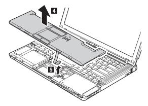
When installing: Make sure that the touch pad connector is attached firmly.
