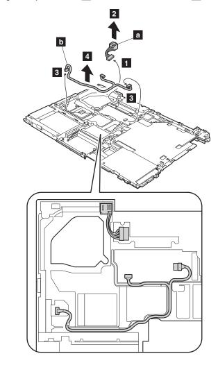
Remove the ac power jack cable **a** and the modem cable **b**.
