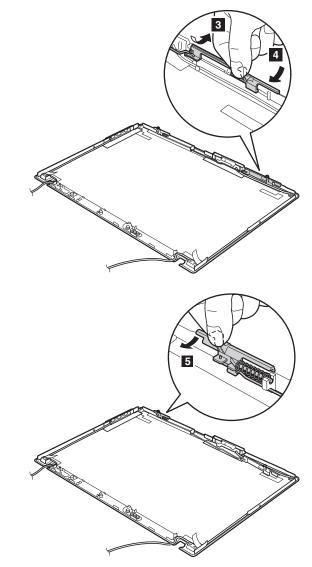
Remove the LCD latches before you remove the antenna cables.
