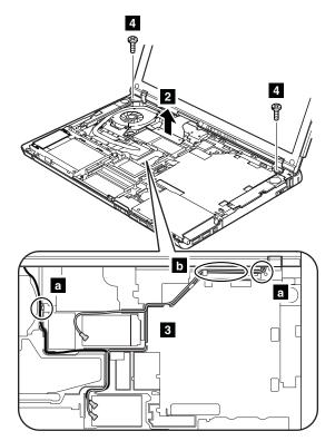
In step **3**, release the antenna cables from the cable guides.
