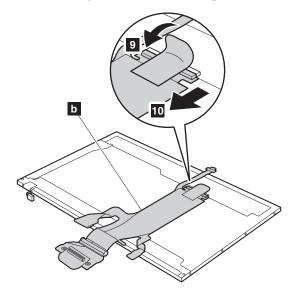
**When installing:** When replacing any LCD FRUs, be sure not to pinch the antenna cables. Make sure that the cables are routed as shown in the figures on page 112 and 113.
