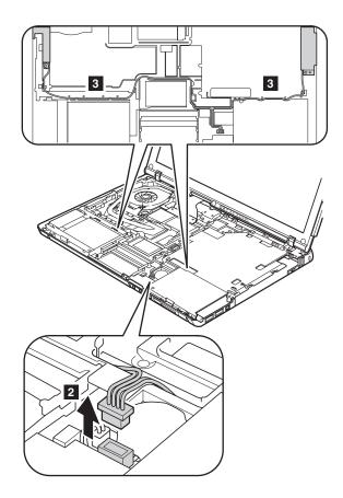
When installing: Make sure that the speaker cables are routed along the cable guides 3 and that the connector 2 is attached firmly.
