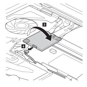
Turn the card over [3], and detach the modem connector [4].
