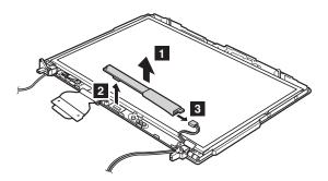
When installing: Make sure that connectors **2** and **3** are attached firmly.
