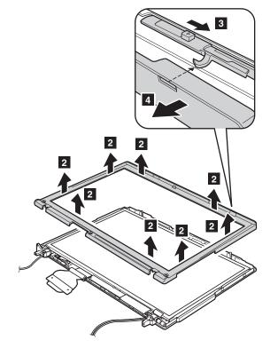
In step **3**, while sliding the LCD latch lever in the direction shown by the arrow, remove the bezel in the direction shown by arrow **4**.
