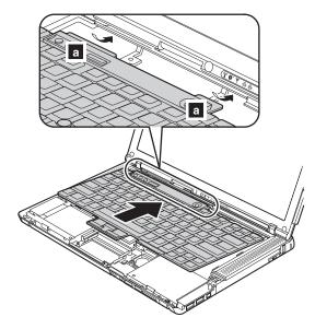
**When installing:** Make sure that the keyboard edges **a** are under the frame as shown in this figure.
