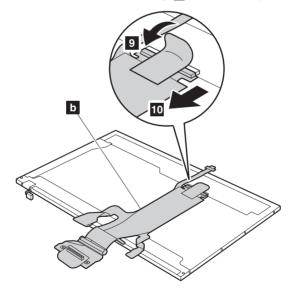
When installing: When replacing any LCD FRUs, be sure not to pinch the antenna cables. Make sure that the cables are routed as shown in the figures on page 131 and 132.
