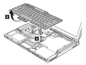
When installing: Make sure that the keyboard edges a are under the frame as shown in this figure.
