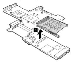
When installing: Make sure that the connector of PC Card slot is attached to the system board firmly.
