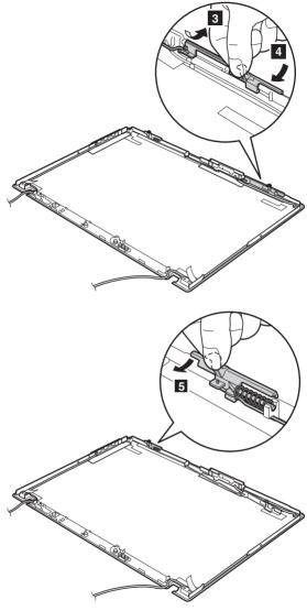
When installing: Attache the latches as shown in this figure.
