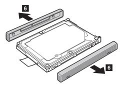
When installing: Rubber rails of the hard disk drive must be attached to the replacement drive. Otherwise the hard disk drive cannot be properly installed to the computer.
