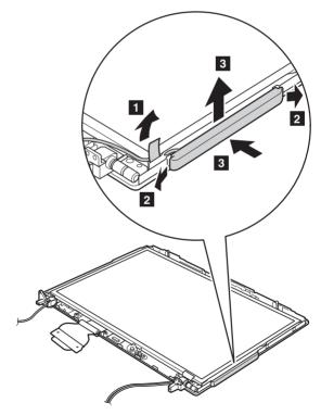
When installing: In step **2**, press the part indicated by the arrow until it snaps into place.
