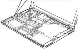
When installing: Make sure that the antenna cable is routed along the cable guides, and that the antenna is attached to the guides a firmly.
