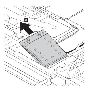
When installing: Plug the gray cable into the jack labeled MAIN on the card, and the black cable to the jack labeled AUX.
