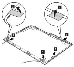
Remove the LCD latches before you remove the antenna cables.
