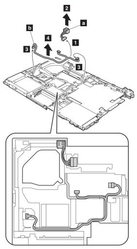
When installing: Make sure that the connectors 1 andare attached firmly, and that the cables are routed as in the figure above.
