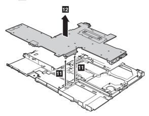
When installing: Attach the system board so that the two small projections on the MG frame 11 fit into the holes provided, and then secure the system board with the screw.
