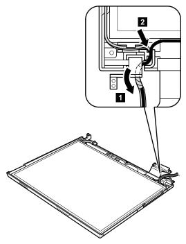
Peel the tape securing the Bluetooth wireless antenna assembly 3.
