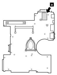
• System board without the security chip (bottom view)
