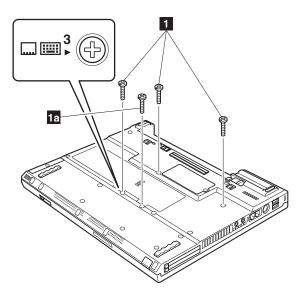
Note: Screw la is only for the models with 14.1-in. LCD. Other models do not have this screw.
