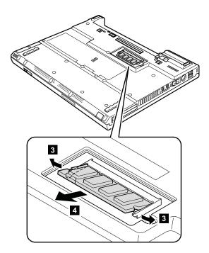
When installing: Insert the notched end of the DIMM into the socket. Press the DIMM firmly, and pivot it until it snaps into the place. Make sure that it is firmly fixed in the slot and does not move easily.
