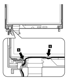
d. Coil the spiral tube round the antenna cables.
