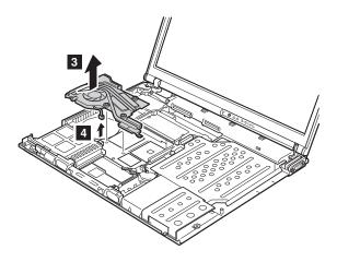
When installing: Make sure that the connector 4 is firmly attached.
