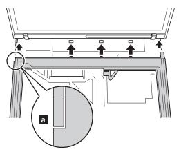
2. Press the left edges **2** and the front edges **3** of the keyboard bezel until the latches are snapped.
