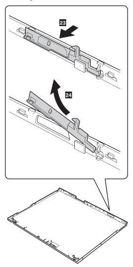
Remove the right latch from the LCD cover.
