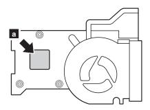
Figure 1. Fan assembly, short
