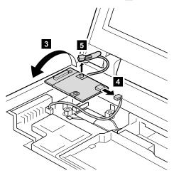
When installing: Make sure that connector 4, the jack5, and the connector on the underside of the card are firmly attached.
