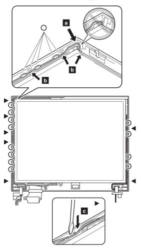
Then route the cables to along the cable guides of the LCD cover. When you route the cables around the LCD hinges, do as shown in  $\cable{c}$ .
