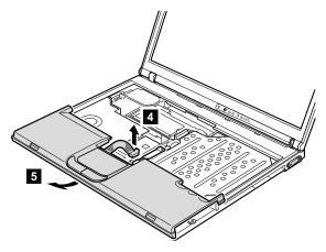
When installing: On a model with a touch pad, make sure that connector 4 is firmly attached.
