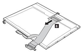
When installing: Make sure that the FPC connector is firmly attached to the LCD panel.
