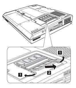
When installing: With the notched end of the DIMM toward the socket, insert the DIMM into the socket, and then press it firmly. Pivot the DIMM until it snaps into place. Make sure that the card is firmly fixed in the slot and does not move easily.
