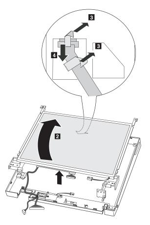
When installing: Make sure the LCD cable is not pinched and aligned to the left of the speaker.
