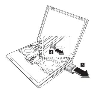
When installing: At steps 2 and 3, tighten the two new screws slowly until both screws have caught the first threads of the screw holes on the PC card slot assembly. Then, tighten each screw one turn at a time, alternating between screws to evenly pull the assembly connector onto the system board connector.
