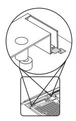
When Installing: Be sure the corners of the FDD cover go under the clasps on the FDD bracket.
