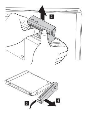
When installing: Make sure that the hard disk connector is firmly attached.
