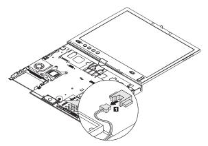
When installing:: Make sure that the speaker cable is firmly connected.
