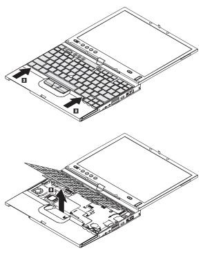
Detach the keyboard connector to remove the keyboard.
