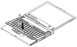
To make sure that the front side of the keyboard is housed firmly, gently press the keys with your thumbs and try to slide the keyboard toward you, shown in the step
