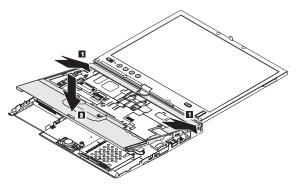
Note: After installing the upper case, route the wireless LAN antenna cable as shown in 3a.
