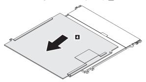
When installing: If digitizer board is defective and needs to be replaced, remove protection sheet from tape before attaching digitizer board to rear side of LCD module as shown. Tpae can be reused if there is no need to replace digitizer board.
