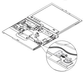
Gently lift upper case up, as shown in step  $\fbox{4}$  and  $\fbox{5}$  , to remove upper case.
