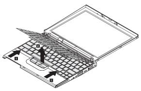
Detach the keyboard connector to remove the keyboard.
