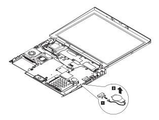
When installing: Make sure that the battery connector is attached firmly.
