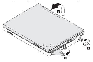
Release the lock knob, shown as 1, and latche knob, shown as 2, to remove the battery pack.
