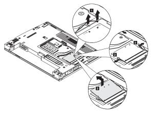
Pull over the levers to detach DIMM.
