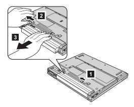
4. Install a fully charged battery.
