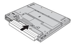
5. Slide the battery latches to the locked positions.
