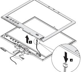
When installing: The replacement bezel should have adhesive pre-applied; therefore, remove the covering from the bezel to explose the adhesive, and then place the top edge under the frame, shown as 1, then push the bezel down and secure with the latches.
