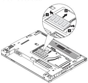
Remove MDC-2 (IBM Integrated 56K Modem).
