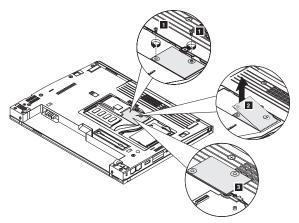
Or remove BMDC-3 (IBM Integrated Bluetooth IV with 56K Modem).
