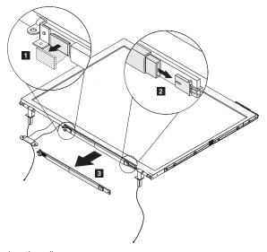
When installing: Attach the inverter back to its original position, as shown in step 1. And reconnect the LCD cable and inverter cable, as shown in step 2. Then secure with the one screw, as shown in step 3.
