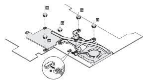
Remove Fan cable then release four screws to remove Fansink for the models with LV processor.
