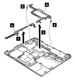
When installing: Make sure that the connectors 2 are firmly attached to the system board.
