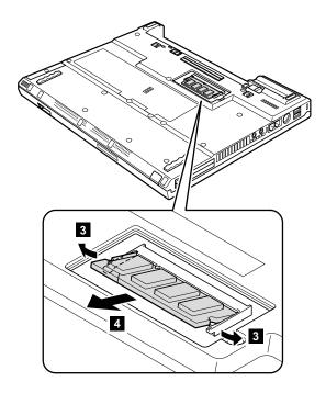
When installing: Insert the notched end of the DIMM into the socket. Press the DIMM firmly, and pivot it until it snaps into the place.
