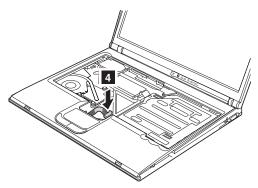
Secure the keyboard bezel from the underside of the computer with the screws b and c.
