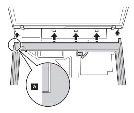
Press the left edges 2 and the front edges 3 of the keyboard bezel until the latches are snapped.
