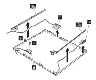
Note: Step **9** is only for the models with the *Bluetooth* wireless features. For the other models, skip this step.
