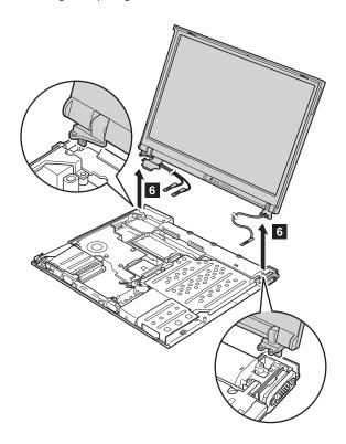
When installing: Make sure that the security keyhole which is on the left-rear corner of the base cover and the keyhole of the bracket inside are aligning firmly.
