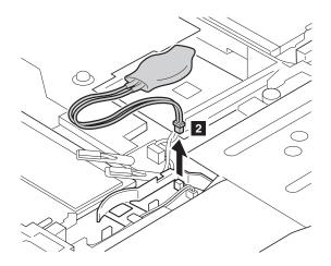
When installing: Make sure that the battery connector 2 is firmly attached.
