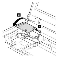
When installing: Make sure that connector 4 and the connector on the underside of the card are firmly attached.
