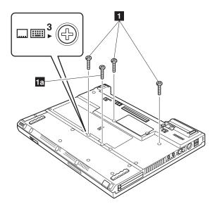
Note: Screw 1a is only for the models with 14.1-in. LCD. Other models do not have this screw.
