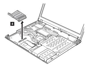
When installing: Make sure that the connector on the underside of the PC Card/ExpressCard slots 2 is firmly attached, and then secure the slots with the screws.
