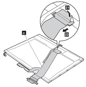
Remove the right latch from the LCD cover.
