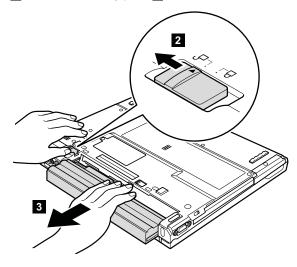
When installing: Install the battery pack along the slide rails on the left and right sides of the battery-pack slot. Then make sure that both battery latches, a and b, are locked, as in the following figure.
