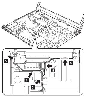
When installing: Make sure that the antenna cables are correctly routed and securely in place.
