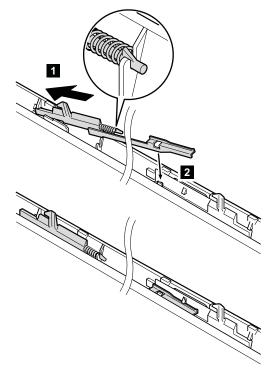
2. Paste three gaskets only for the models with *Bluetooth* wireless features. For the other models, skip this step.
