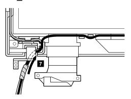
Move the spiral tube until it reaches at the cable guide of the LCD cover as in this figure. Make sure that the antenna cable is not pinched by cable clip ( a ).
