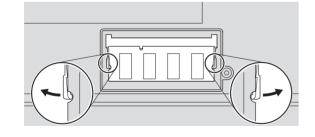
Verify proper installation of the optional SO-DIMM:
