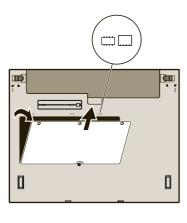
**7** If a SO-DIMM is already installed, remove it as shown. Save the SO-DIMM for future use.
