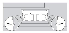
Align the notch in the contact edge of the SO-DIMM with the divider in the socket. Firmly insert the SO-DIMM into the socket at an angle of 20 degrees 1, and then pivot it downward until it snaps into place 2.
