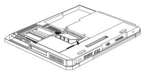
Note: When you install the PCI card, remember to insert it into its socket at 20°, press it down and ensure the connection is well.
