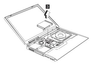
Note: Before removing and replacing the PCMCIA holder, make sure that the PCMCIA cards are removed and the eject levers are sticking out.
