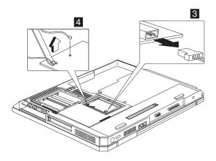
Note: There are 2 cables on step 4: The gray cable is the main antenna and the black cable is the auxiliarey antenna. There is no step 3 if the Mini-PCI card is not stalled, then this cable will be connected to the
