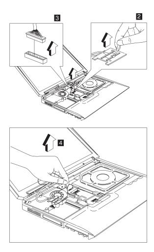
**Note:** Release the gray cable, which is the main antenna from the system.
