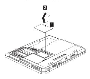
Note: The screw does not separate from the PCI cover.
