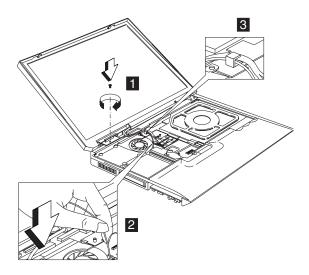
**Note:** Please follow number 1, 2, 3 to reintsall the auxiliary antenna and arrange the cable well based on the above drawing.
