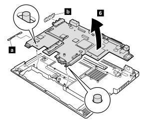
When installing: Attach the system board so that the two small projections on the base cover fit into the holes provided, and then tighten the screws.
