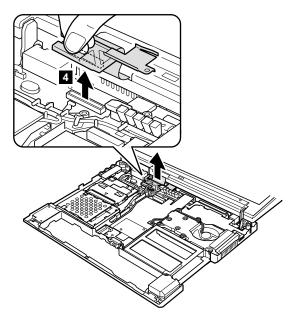
When installing: Make sure that the connector 4 is firmly attached.
