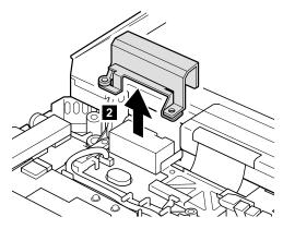
When installing: Attach the hinge cover, aligning the two projections on the rear side with the two small square holes in the base cover. ( a )
