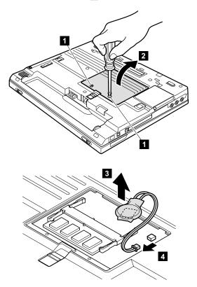
When installing: Make sure that the battery connector is attached firmly.
