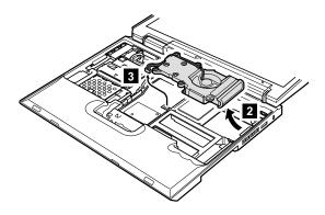
When installing: Make sure that the connector **3** is firmly attached.
