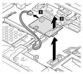
When installing: Make sure that connectors **2** and **3** are attached firmly.
