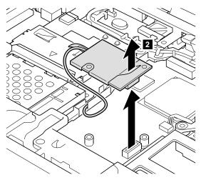
**Note:** When unplugging the Bluetooth antenna jack, do not pull the cable; it might snap. Unplug the jack by pulling the tab with your fingers.
