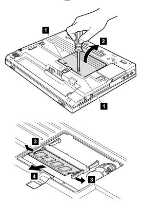
When installing: With the notched end of the DIMM toward the socket, insert the DIMM into the socket, and then press it firmly. Pivot the DIMM until it snaps into place. Make sure that the card is firmly fixed in the slot and does not move easily.
