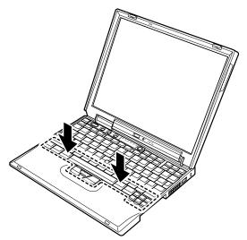
To make sure that the front side of the keyboard is housed firmly, gently press the keys with your thumbs and try to slide the keyboard toward you.
