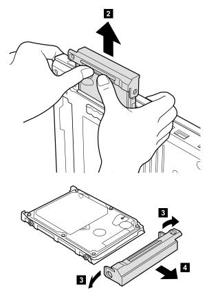
When installing: Make sure that the hard disk is connected firmly.
