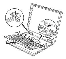
2. Align the tabs of the keyboard with the corresponding slots; then press the keyboard until it snaps into place.
