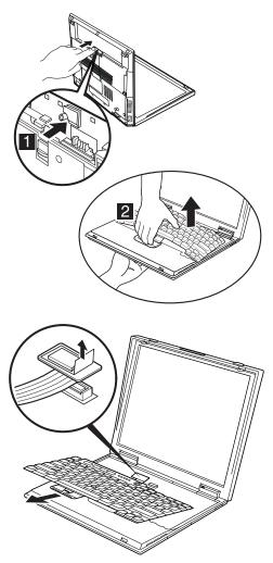
When installing: When installing the keyboard, do as follows:
