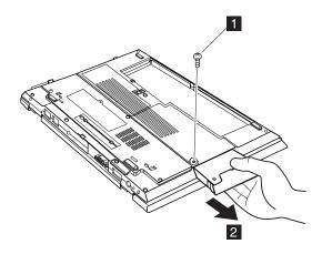
Note: The hard disk is attached to the cover.
