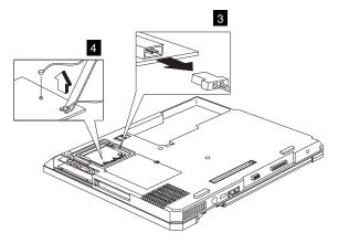
Note: There are 2 cables on step 4 : The gray cable is the main antenna and the black cable is the auxiliarey antenna.
