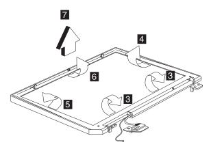
Note: When removing the LCD, take note of the following:
