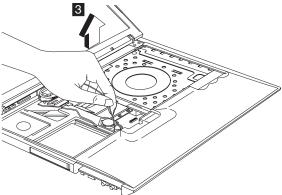
**Note:** Release the gray cable, which is the main antenna from the system.
