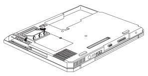
Note: When you install the PCI card, remember to press it down and ensure the connection is well.
