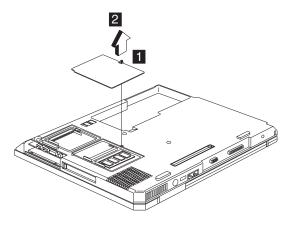
Note: The screw does not separate from the memory cover.
